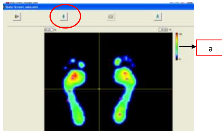
Figure3.2: Force distribution under the foot in the static position, a shows the magnitude of pressure distribution.
