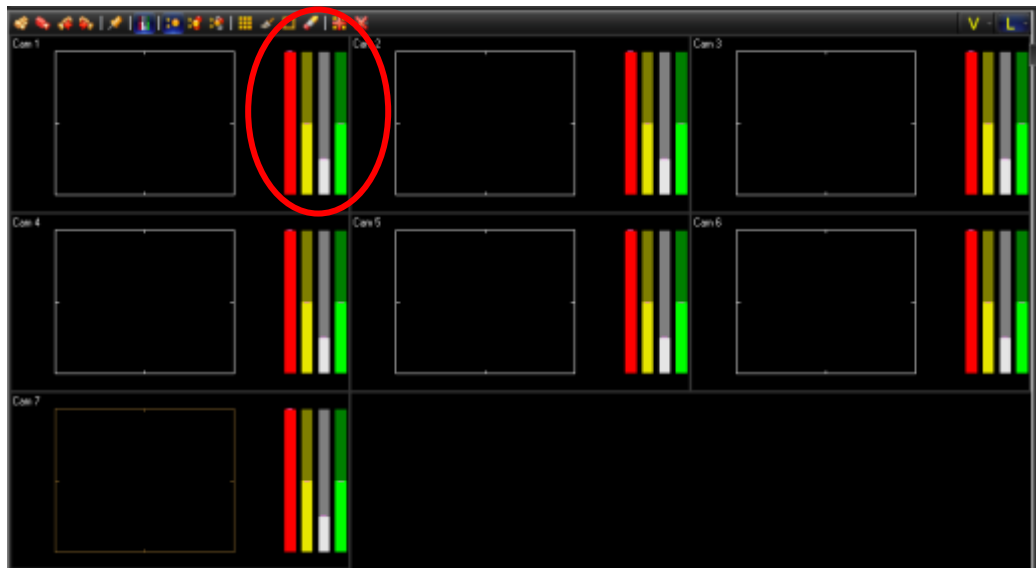
Figure3.11: The views of the seven cameras. The bar graphs beside each camera represent the hardware setting attributes. Key: red represents strobe intensity, yellow shows threshold, gain shows white and circularity shows green.
