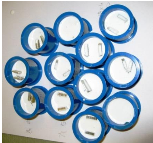
Figure 60 A batch of samples being casted prior to polishing
