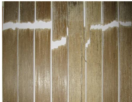
Figure 56 Examples of a trial hemp reinforced unidirectional samples fracturing at the edge of the grip area. Stress concentration created by grips causes premature sample fracture and invalidity
