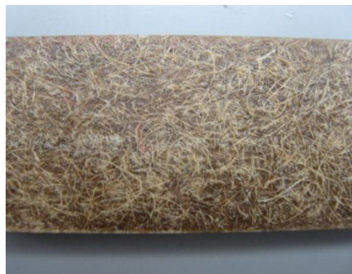
Figure 86 Surface of the hemp mat (HM) reinforced Palapreg-eco resin laminate
