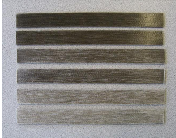
Figure 91 250Tex non-twisted fibre flax yarn laminate strips with different volume fractions ( From the top: 23.0%, 30.0%, 51.0%, 56.6%, 76.0% and 89.7% V_f .)
