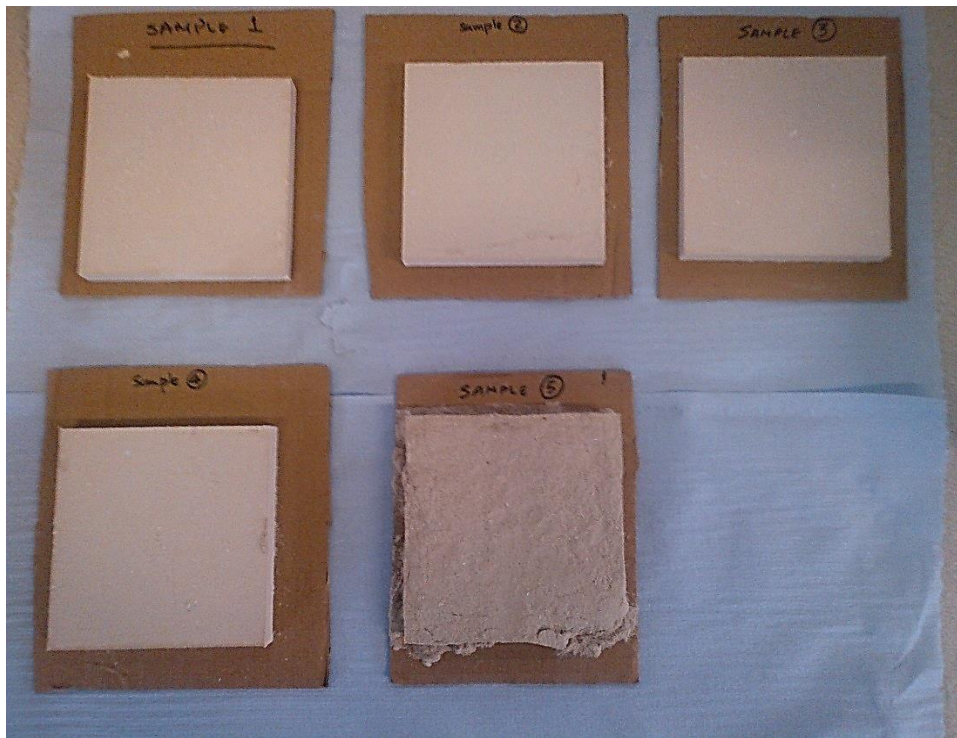
Figure 4.3 Core boards samples (100 mm × 100 mm) 1-3 (Top left to right) and 4-5 (Bottom left to right) placed on cardboard pieces
