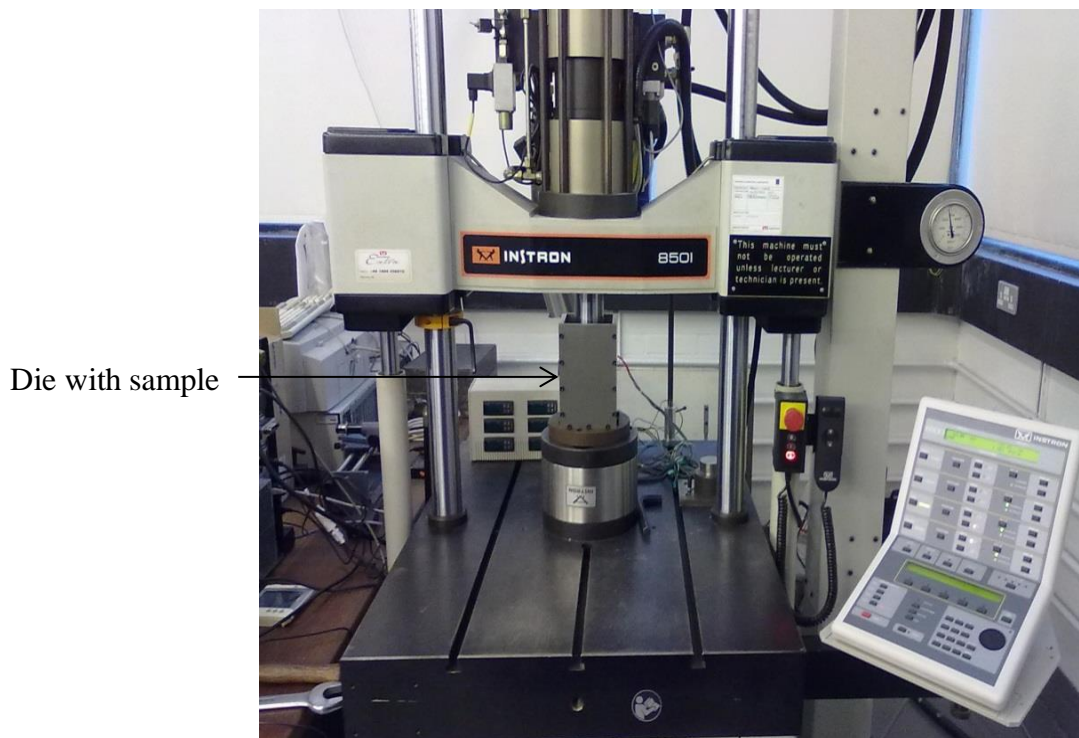
Figure 3.9 Compaction of core boards using INSTRON 8501 Test Machine
