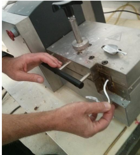
Figure 5-2: Twin screw extrusion of the composite material
