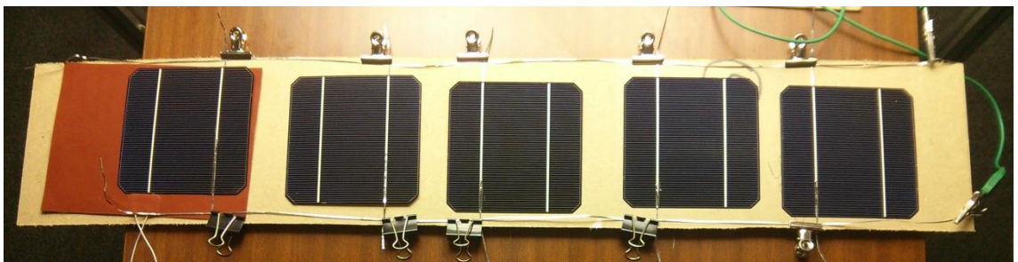
Figure 4-48: Experimental testing of output voltage for four cells connected in parallel.
