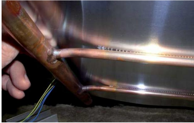
Figure 4-27: Separation of laser welded pipes on similar absorber. Source [104]
