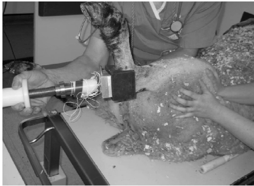
Figure 117: Axial compression test equipment being tested on an ovine leg
