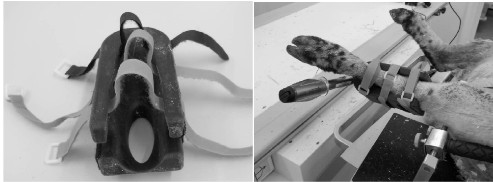
Figure 115: Orthotic shoe with velcro straps design by S&N Memphis to simulate and apply the torsion on the ovine leg
