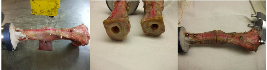
Figure 128: Pictures illustrating the excised bone before and after sectioning along the original fracture line
