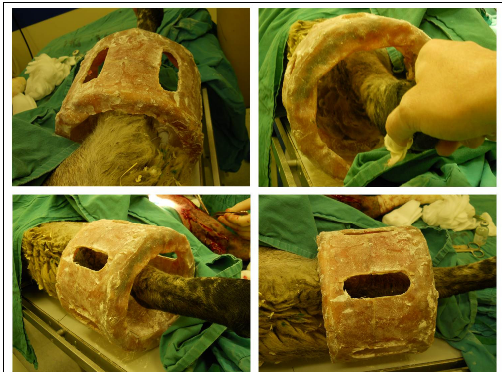
Figure 111: The glass reinforced polymer housing being trialled on its own on an ovine model left hind limb
