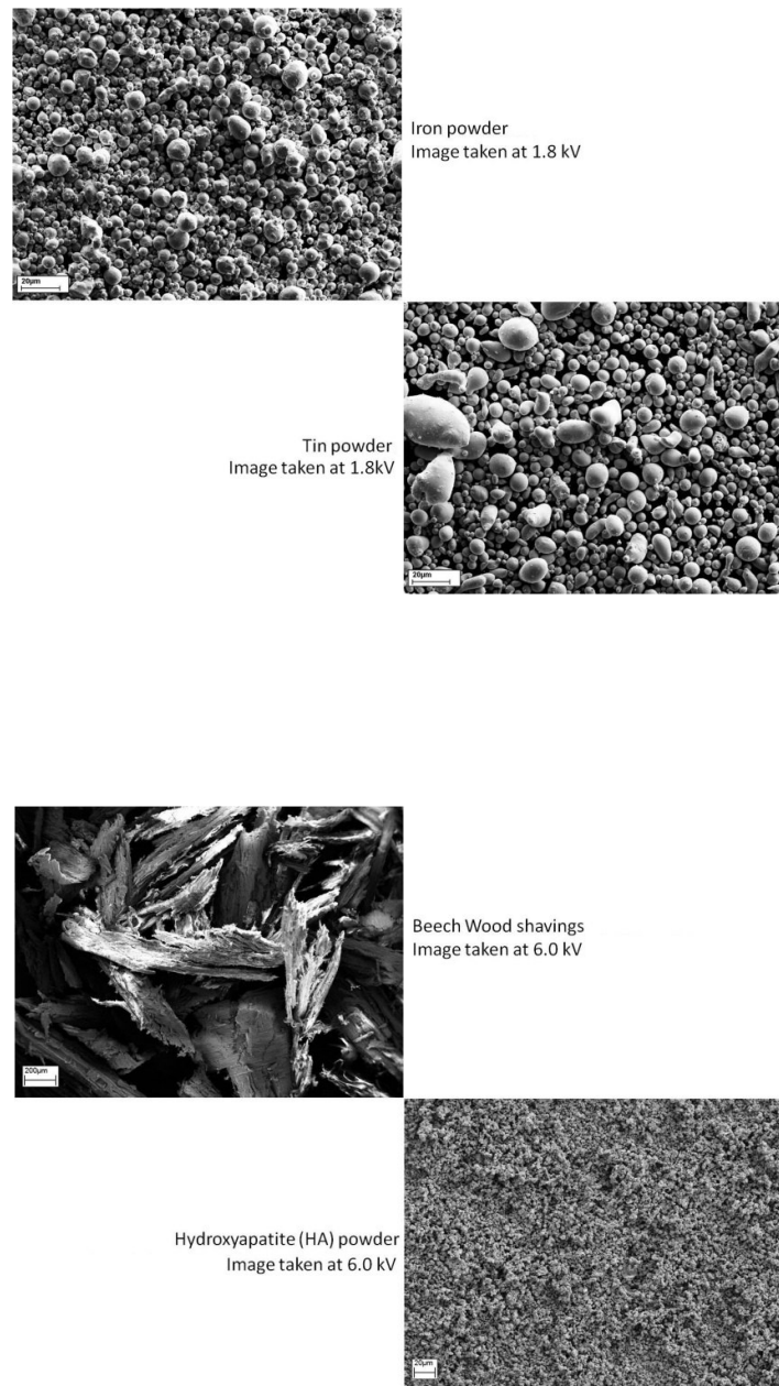
Figure 22: SEM images of selected particulates for callus composite
