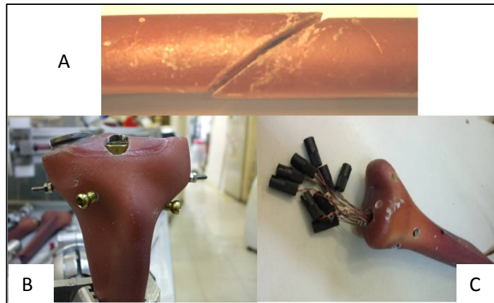
Figure 26: Figure A shows the fracture induced replicating 42 A2 fracture; B shows the proximal part of the tibial bone with the nail inserted and the screws in place; C shows the distal end with the wires from the instrumented nail exiting
