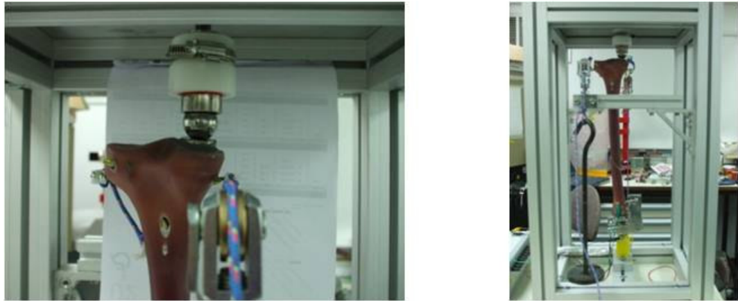
Figure 31: Left picture shows the loading contact point for axial compression and the right picture showing the pulley system for the internal and external torque
