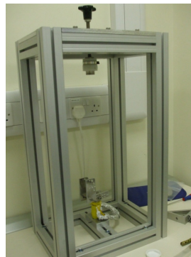
Figure 28: Custom made aluminium frame for axial compression and torque testing
