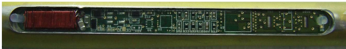
Figure 120: Instrumented pocket of GEN III Nail
