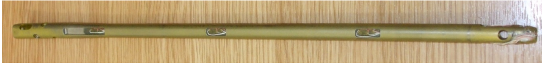
Figure 24: GEN I showing the pockets on the anterior side of the nail
