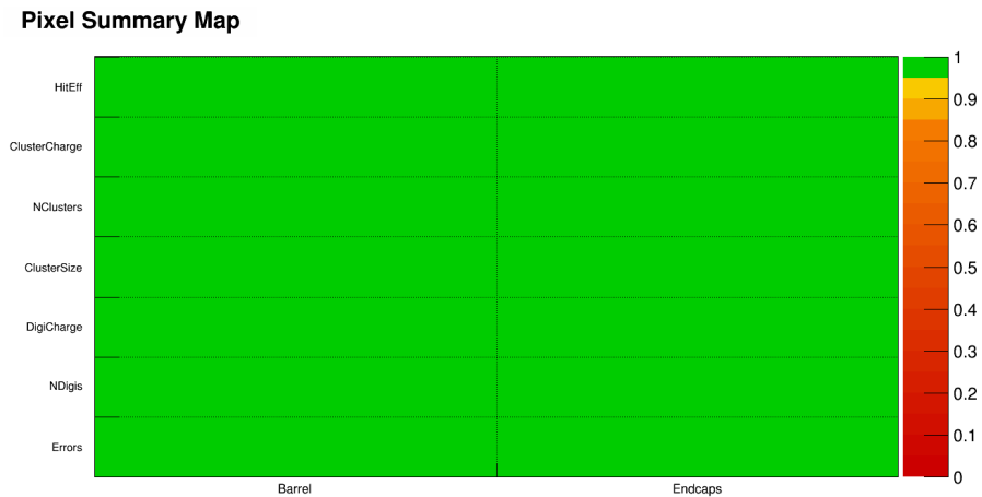
FIGURE 4.3: The summary map for the pixel detector as seen in the DQM GUI. The map is divided along the x-axis into barrel and endcap, and along the y-axis by the chosen quality tests. A green square indicates nominal values for the relevant quality test, whereas a red box would indicate an error flag set. An orange box indicates a warning flag.
