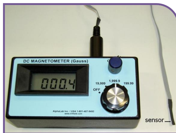
Figure 4.17: The magnetometer used to measure the magnetic flux density of permanent magnets
