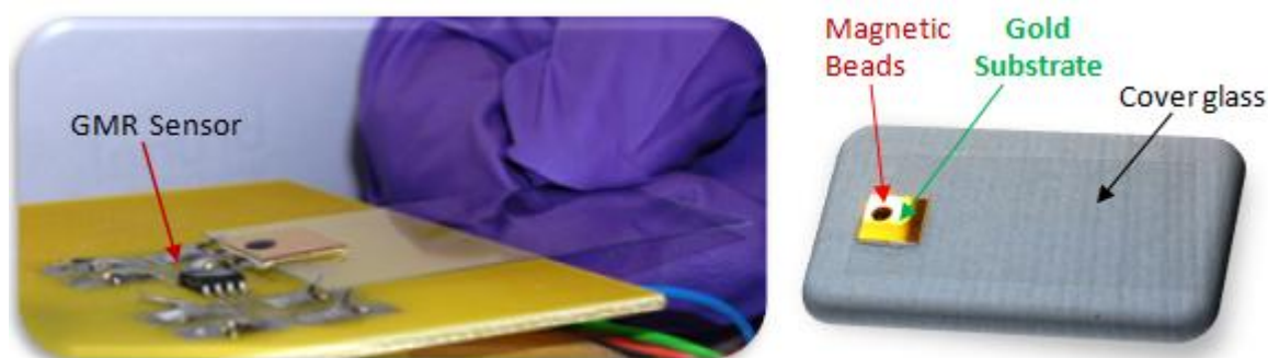
Figure 6.7: Magnetic beads on gold substrate applied to the GMR sensor
