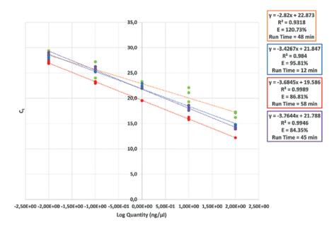
Figure 1. Amplification efficiency of four qPCR instruments; CFX96 (green), xxpress (blue), ABI Prism 7900 HT (red) and Rotor-Gene Q (purple).
