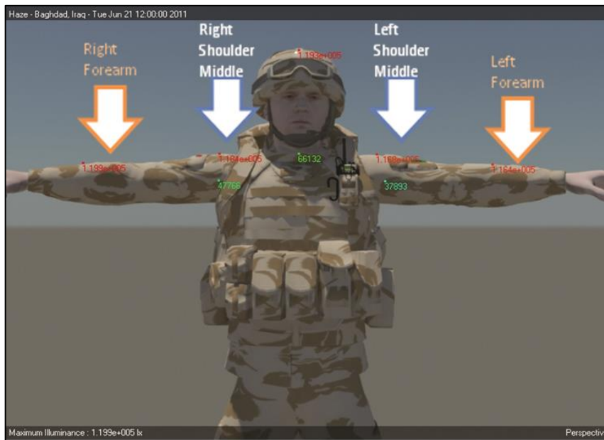
Figure 14 The positioning of the virtual light sensors (front)
