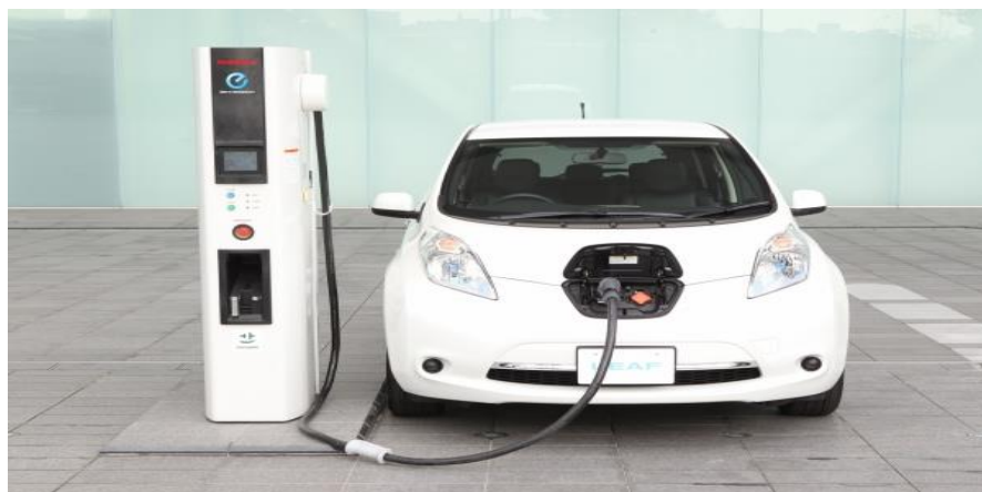
Figure 2. 23: DC Fast Charging Station from Ecotricity connected to Nissan Leaf [29]
