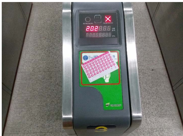
Figure 8. RFID card and reader of Daejeon subway paying system
