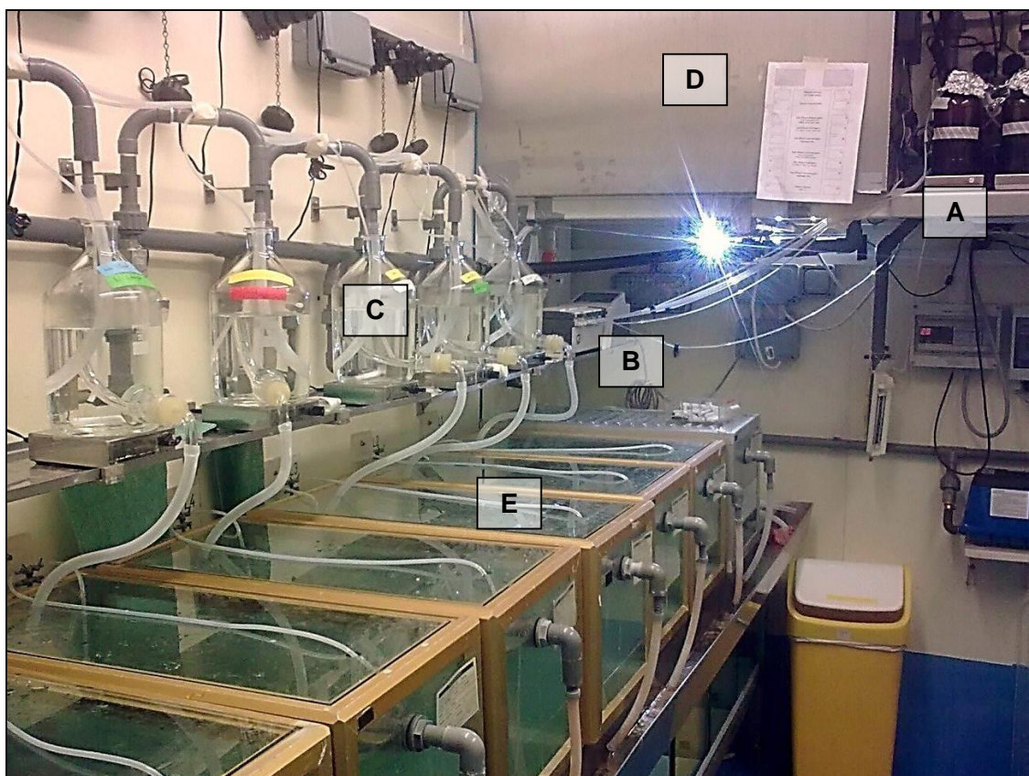
Figure 3.2 The experimental set up for dosing exposure tanks. Solvent carrier from chemical stock bottles (A) was pumped through silicone tubing via peristaltic pump (0.01 mL/min) (B) to aspirator bottles (C), where it was diluted in aquarium water from the header tank flowing at 30 L/hour (D). This produced the desired experimental concentrations which flowed down to the exposure tanks (E) via silicone tubing.
