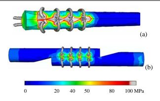
Fig. 5. FE stress analysis result of the sutured tendon under tensile test. The colours define the level of Mises stress on the suture and tendon.
