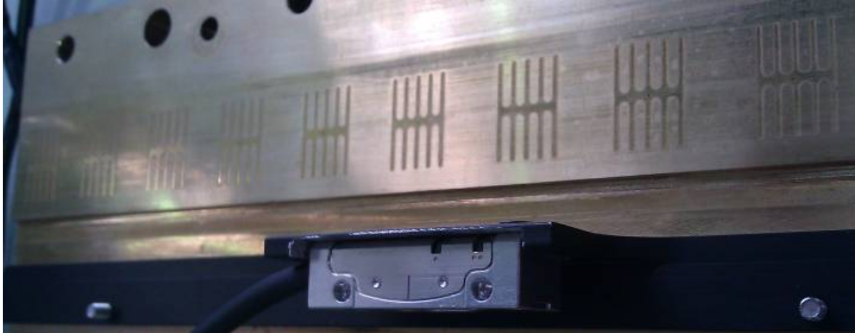
Figure 5-6: Picture of the groove pattern machined in the inner surface of the pressurized bearing to improve stability. The encoder read head can also be seen.
