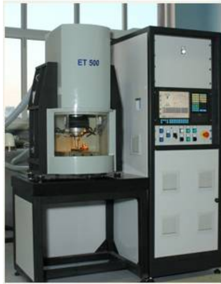
Figure 2-5: Typical ECM machine from Indec. Die sinking only. Source: http://www.indec-ecm.com/en/equipment/ET500/
