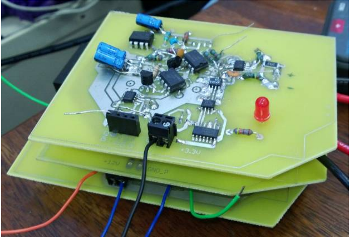
Appendix 4 Figure 24: Picture of the fully assembled first PSU prototype
