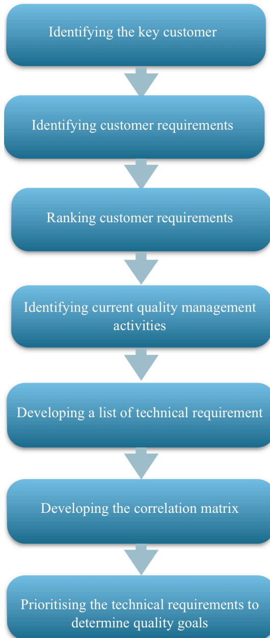
Figure 3-4 QFD as a process. Adopted from: Lim et al. (1999) and Zhanga & Awasthi (2014)
