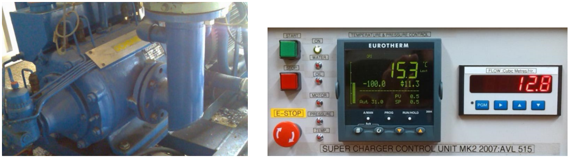
Figure 3.18 AVL Supercharger and its Remote Controller
