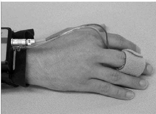
Fig. 3.13: The fitting of an infrared photoplethysmographic cuff to the finger of the subject’s hand allows a continuous non-invasive measurement of arterial blood pressure. (Reproduced from Bogert & van Lieshout 2005).
