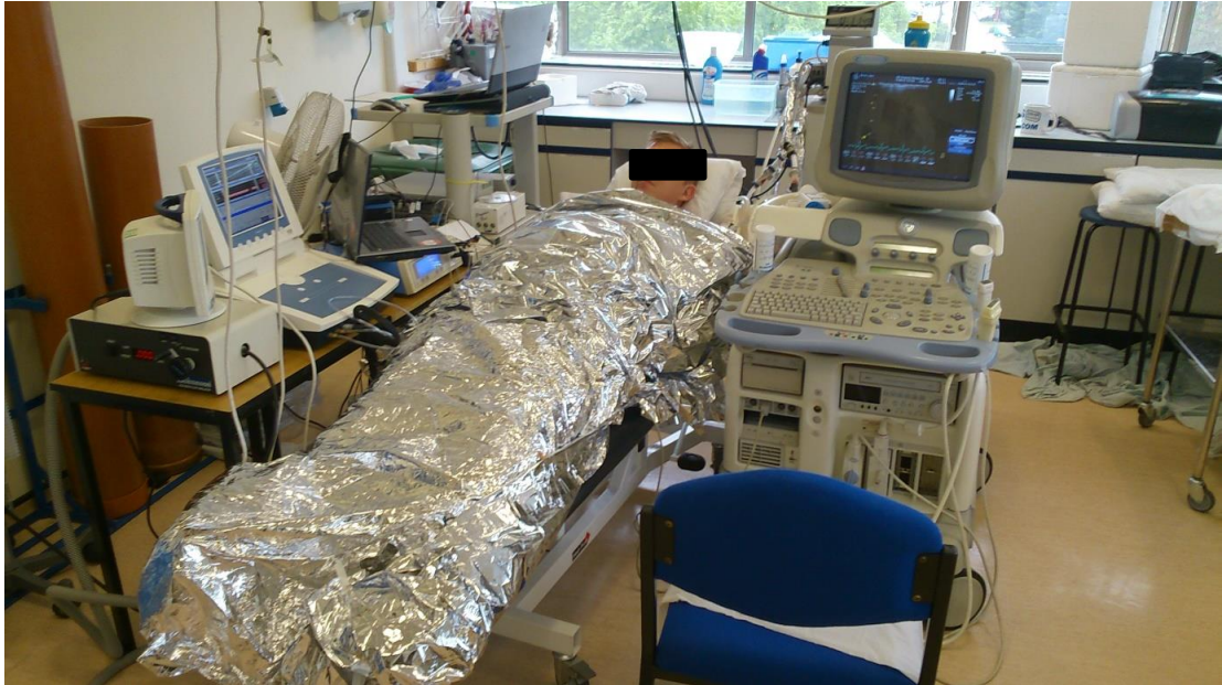
Figure 7.1: Experimental set-up showing subject resting in supine position while core and skin temperatures are elevated through the use of a water-perfused suit.
